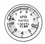
Pressure (lbs/inch<sup>2</sup>) x Cylinder area (inch<sup>2</sup>) = Force (lbs)
